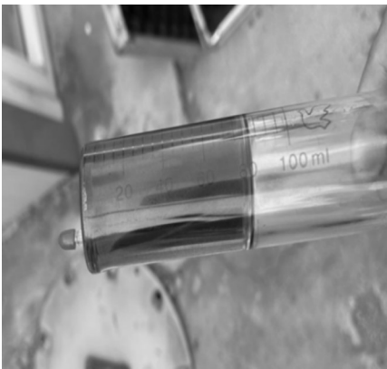
图 12 绝缘油呈棕黑色 Fig. 12 Brown and black of insulation oil
